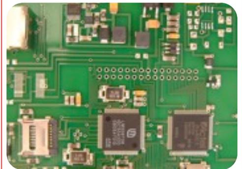
The DDU has powerful onboard processing capabilities, including an FPGA and micro-processor. These allow for complex parallel processing of data in real-time such as Digital Signal Processing while writing to an onboard uSD memory card.
